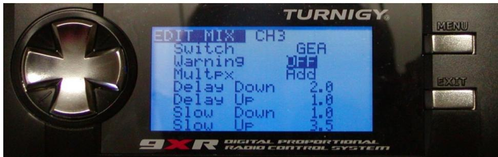
We now have a mix line in the elevator channel, using the throttle switch as the source, which gives 5% down to compensate for the extra lift generated under power. We have a 1 second delay before the elevator compensation starts and a 3.5 second period for it to reach full deployment. At throttle off, we have a delay of 2 seconds while the model slows and then a 1 second period during which the elevator resumes the neutral position for the glide.
