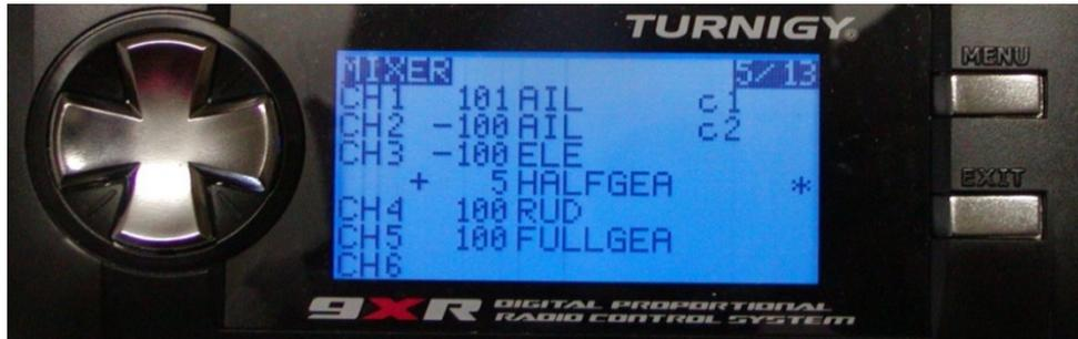
When the GEA switch is flipped to ON, the signal to the ESC via CH 5 goes from -100% to +100% because that's how the FULL input works: the value is either -weight or +weight.
