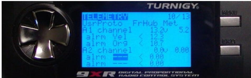
The first item on the page is 'UsrProto', where you select between WSHhi (*Winged Shadow How Hi*), FrHub (*FrSky Telemetry Hub*) and DSMx (*DSM2 or DSMX Telemetry*). On the same line you can select either Metric or Imperial units.
