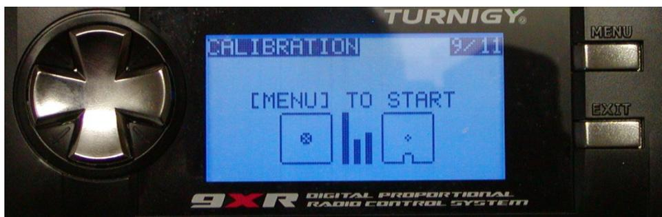
NOTE: It is **essential** to calibrate the transmitter initially and whenever there are any changes that could affect the stick or pot outputs (e.g., replacement of a stick assembly). With the 9XR Pro (unlike the 9XR) the calibration data are stored in General Settings, separate from model memories.
