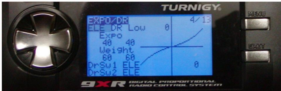
For each control you can set two switches. For a dual rate arrangement, simply chose the appropriate switch (say ELE) for DrSw1 and leave DrSw2 blank. To have the switch work in the reverse direction, choose the “not” form (!ELE).
