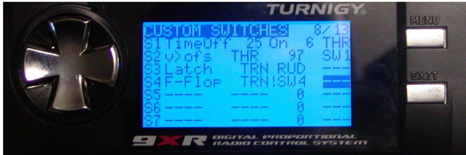
The **Latch** function allows a state or event to be captured and held for as long as required. For example, the maximum altitude reached by a glider can be retained until it is desired to measure a new maximum.
