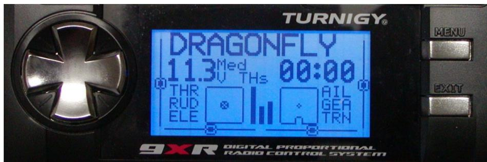
In the upper half of the screen, the transmitter voltage is displayed in large print, along with the trim increment type, here 'Med' (see page 20). The current value of Timer 1 is also shown in large print, along with the switch used to activate it, here 'THs' (see page 19). In addition, the current Flight Mode will be displayed if it is other than the default FM01.
