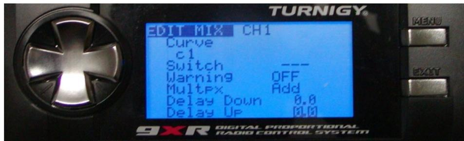
5. **Curve:** This applies a function or curve to modify the application of the source value.
