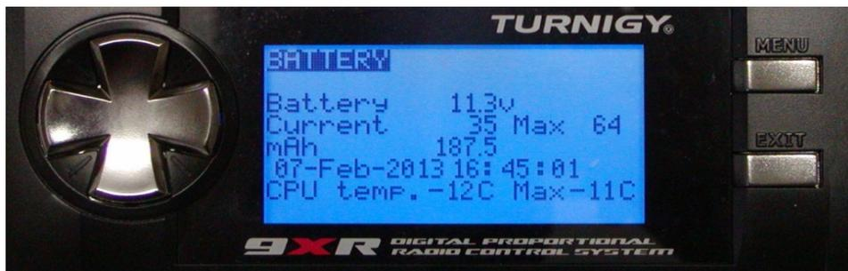
The mAh reading shows the battery capacity used since the last reset, normally after charging the battery. To reset the number to zero, long press the MENU key. To adjust date or time, go to page 6/11 of the Radio Setup screens.
