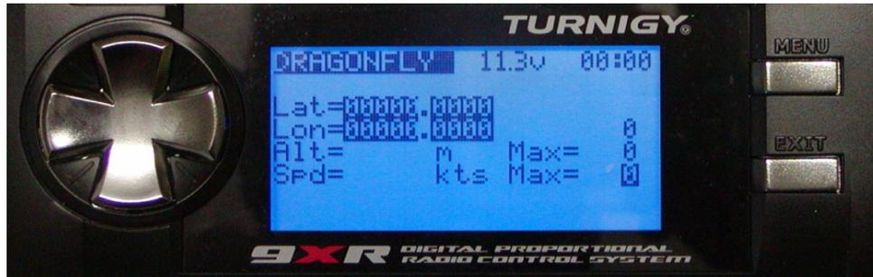
A long press of the MENU button will reset the maximum altitude and maximum speed readings to zero. For further information on telemetry see page 36.
