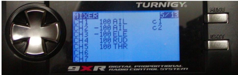
The various channels numbered on the left of the screen are outputs from the mixer to the servo. For example CH1 is servo slot number 1 on your receiver. CH2 is servo slot number 2, and so on.
