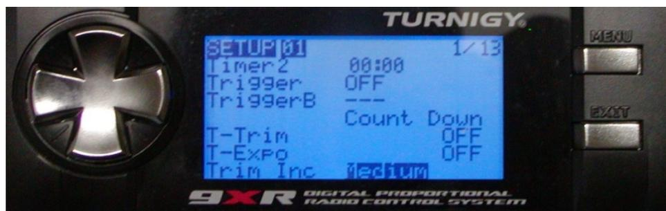
Trigger B options are any physical switch or any virtual switch (more on those later). Both A and B switches can control either count up or count down.
