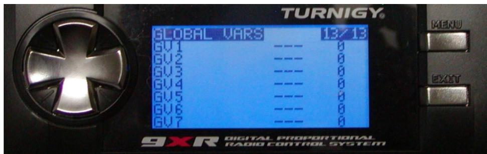
For example, to use a global variable in the EXPO/DR menu, highlight the Expo or D/R value and then long press MENU key. You will then have the ability to select GV1 through to GV5. Then in the GLOBAL VARS screen (above) define the GVx, which you chose to be any of the potentiometers, P1, P2 or P3. Go back to the EXPO/DR screen. As you adjust the potentiometer, the value of the Expo changes and the shape of the graph changes.
