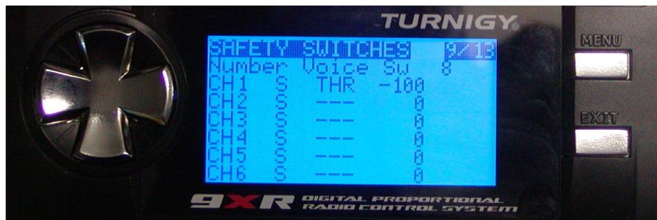
Warning! When a safety switch is active, the output of the channel is replaced by the defined safety switch value (here -100). The value of the channel, however, continues to be determined by the throttle stick position (and any other mixes that feed into it). If you were to have a mix to feed in down elevator in proportion to the throttle setting, cutting off the motor at full throttle with the safety switch would leave the elevator still in its down position.
