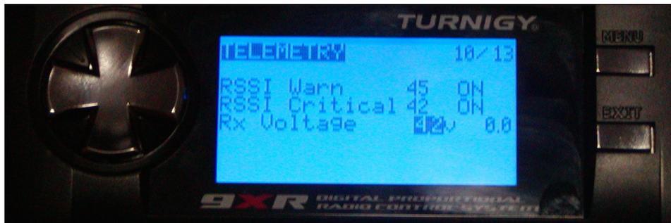
Similarly audio alarms will be triggered at "warning" and "critical" levels if the received signal strength indication (RSSI) or the receiver voltage falls below the set levels. These settings, at the bottom of the Telemetry page, are shown above.
