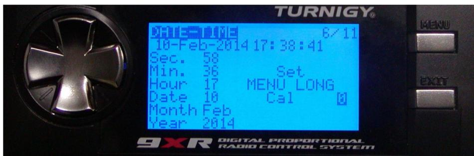
The calibration (Cal) value may be changed to correct inaccuracies in the clock.
