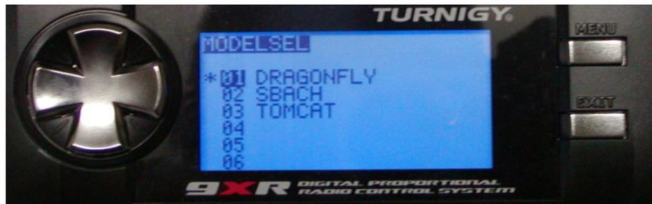
Once a model slot has been highlighted, SELECT, COPY, MOVE, DELETE and BACKUP commands become available, as shown below. Move the cursor using the UP or DOWN key and pick the option by pressing the MENU key.
