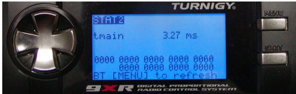
The screen also shows information relating to the BIND reply if a DSM module is used and 'BT reply' (Bluetooth), if the necessary hardware is installed. Another short press of the UP key brings you back to the home page from whence you started.
