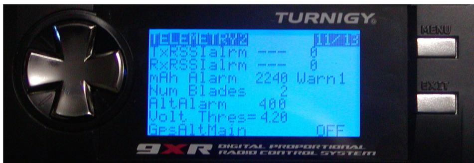
**RSSI Alarms:** TxRSSIalarm and RxRSSIalarm refer to the levels at which warning beeps are produced directly by the FrSky module (see page 10). The numbers here are read from the transmitter module. If you have modified a FrSky DJT module in accordance with the instructions in the manual *Introduction to the Hardware*, these numbers may not appear. They are normally set to zero (turned off), as shown above, to avoid conflict with the RSSI alarms set on the Telemetry page,.
