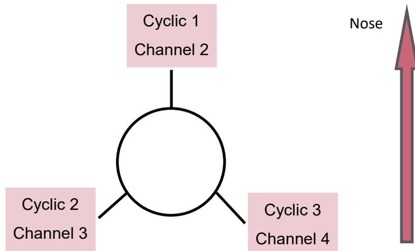
1. Ensure the horns are near 90 degrees when at mid stick. (TH has linear pitch curve and you can use the monitor screen to ensure the transmitter is putting out 0 on Aileron, Elevator and Pitch channels). We can sub-trim them after mix correction is finished.
