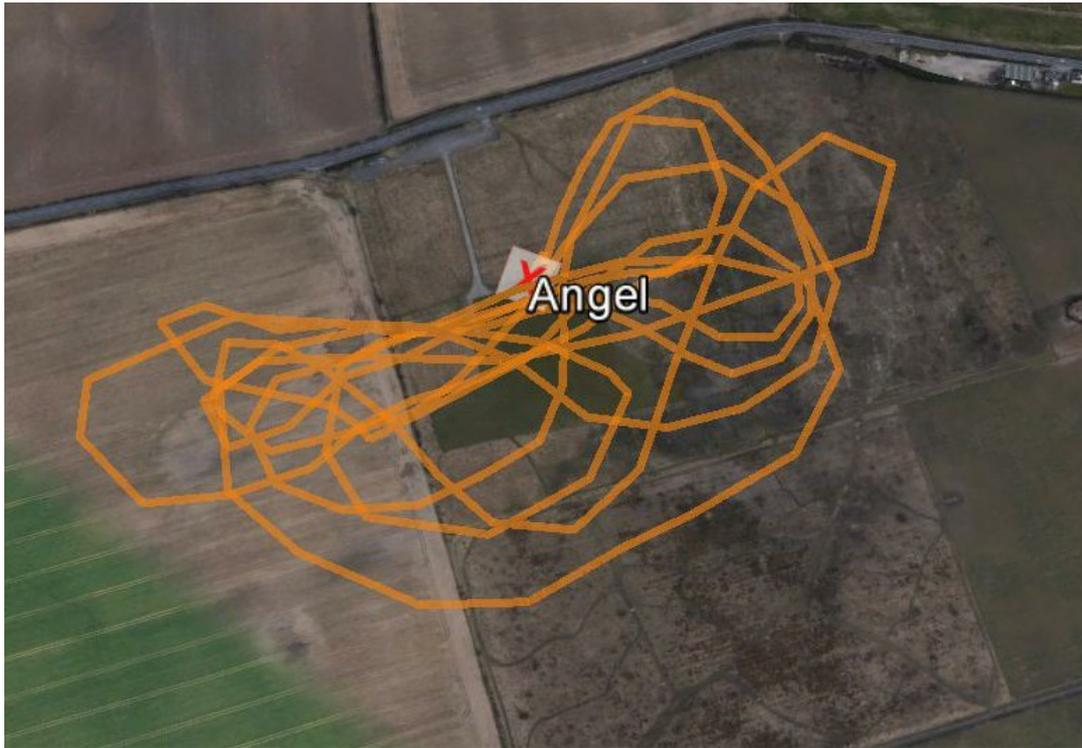
Provided one has GPS logging data, clicking on the Google Earth button will automatically plot the flight. The name of the plane is shown, in this case Angel, and the flight path recorded. Ample proof for the club Safety Officer that I did not fly over the road with my plane! By altering the Google Earth perspective, different views can be obtained.
