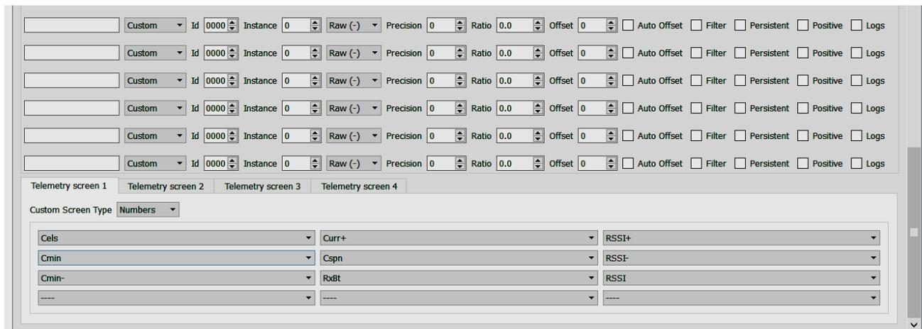
First select the telemetry screen, then the custom screen type, then any of a whole range of parameters can be entered into the screens. This is probably the last operation to set up once a model has been programmed, as it can contain a range of parameters including logical switches, and telemetry values.
