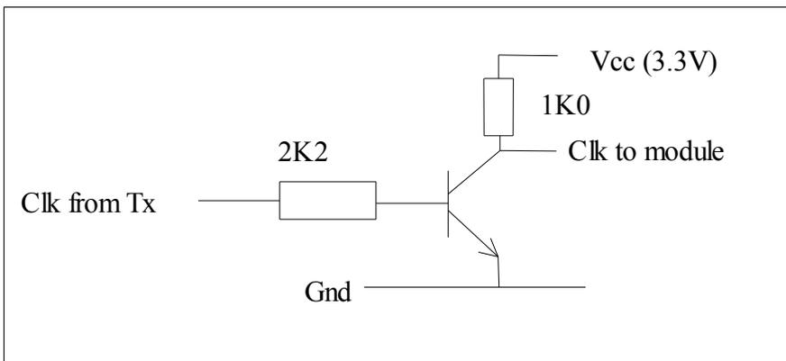
Note that the SKY board has a real RS232 driver, so you need a resistor in the base of the transistor (any general purpose NPN type). The driver outputs +/- 6V which is why the transistor is needed.
