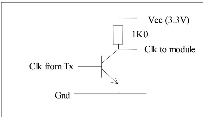
Note that there is a resistor internal to the 9Xtreme, so you don't need a resistor in the base of the transistor (any general purpose NPN type). The resistor actually stops the 9Xtreme from driving the signal fully, which is why the transistor is needed.
