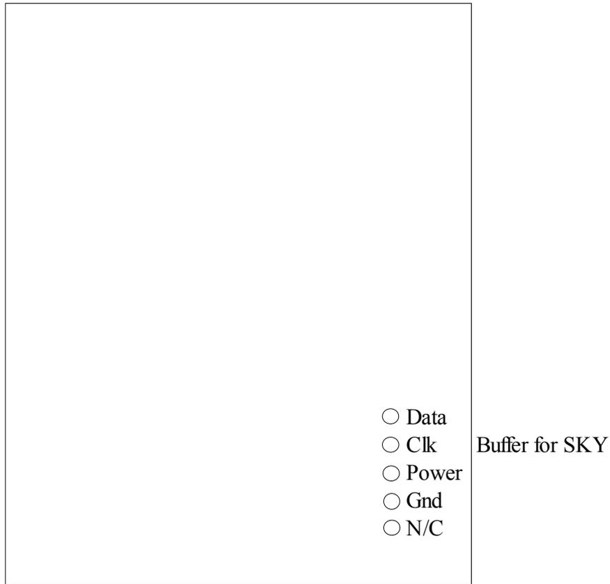
Note that the Power connection is battery voltage, do NOT use this directly to the 3.3V connection on the module.
