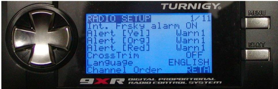
Individual sounds may be set for the three levels of alarm relating to the RSSI values the FrSky receiver telemetry is sending back to the transmitter.
