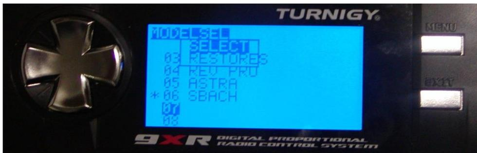
Backup files are saved on the SD card with a “.eepm” extension in a folder called MODELS. They can be copied to the computer via USB (see *Communicating with a Computer*).
