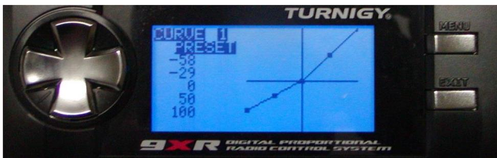
You will see 5 or 9 editable points with the values initially set a zero. Scroll through the points with UP/DOWN. Change the value with LEFT/RIGHT.
