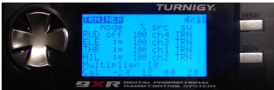
The ‘mode’ column selects how PPMin is used when the Trainer Switch is activated:
