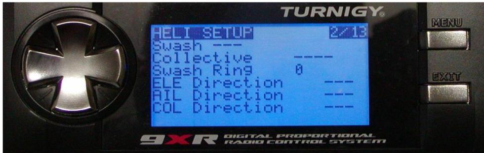
The inputs to the CCPM mixer are the AIL and ELE sticks, plus the input or virtual channel selected in "Collective" (which has entries on the MIXER page for one or more pitch curves). Here are the details:
