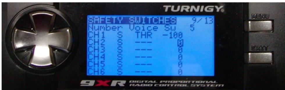
Warning! When a safety switch is active, the output of the channel is replaced by the defined safety switch value (here -100). The value of the channel, however, continues to be determined by the throttle stick position (and any other mixes that feed into it). If you were to have a mix to feed in down elevator in proportion to the throttle setting, cutting off the motor at full throttle with the safety switch would leave the elevator still in its down position.
