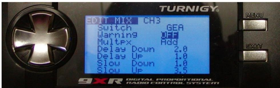
We now have a mix line in the elevator channel, using the throttle switch as the source, which gives 5% down to compensate for the extra lift generated under power. We have a 1 second delay before the elevator compensation starts and a 3.5 second period over which it is fully deployed. At throttle off, we have a delay of 2 seconds while the model slows and then a 1 second period during which the elevator resumes the neutral position for the glide.
