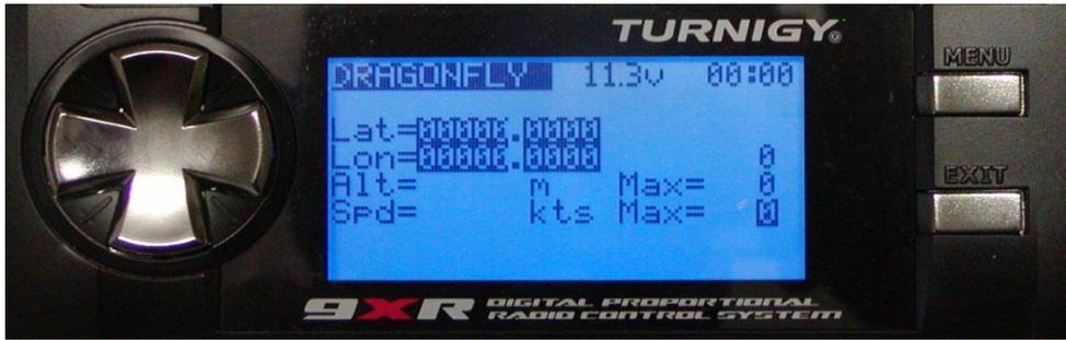
In the picture above, along the top is the model name, battery voltage and timer value. The other values come from sensors in the aircraft and give the GPS latitude, longitude, altitude above the starting point, current speed, maximum altitude and maximum speed since the radio has been turned on. A long press of the MENU button will reset the maximum altitude and maximum speed readings to zero. For further information on telemetry see page 33.
