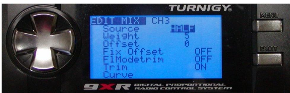
On the ground with motor disconnected, check that the elevator compensates in the correct direction (down). If not, invert the weight to minus 5. (i.e., just highlight the number and press both the RIGHT and LEFT keys simultaneously).
