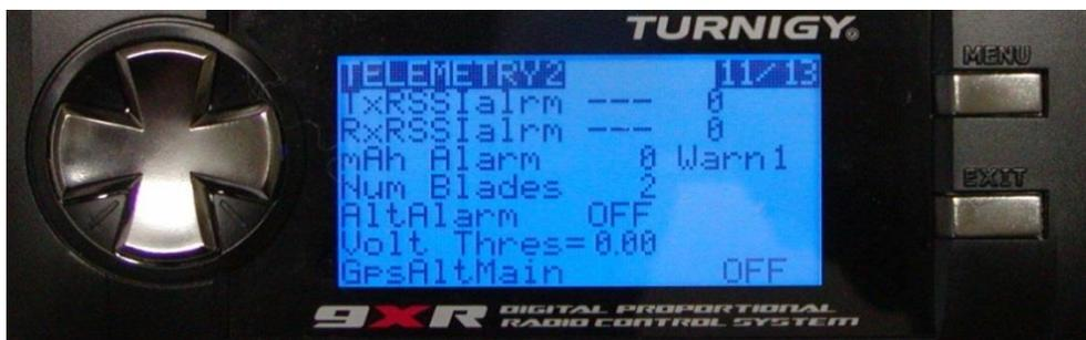
**Alarms:** "Low" and "Critical" alarms for RSSI and the mAh Alarm will trigger audio warnings when the measured value goes below the defined levels. When a Micro-SD card with voice files is present in the slot, those alarms will be announced by voice (e.g. "RF signal Low"). If no card is present each will trigger a different beep pattern.
