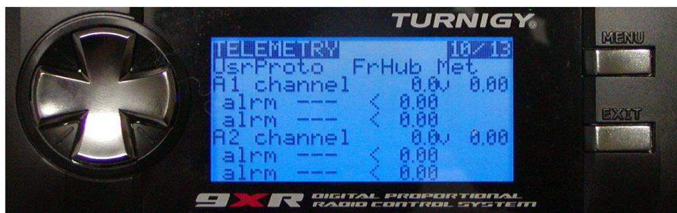
'UsrProto' is where you select between WSHhi (*Winged Shadow How Hi*) or FrHub (*FrSky Telemetry Hub*) and between Metric and Imperial units.
