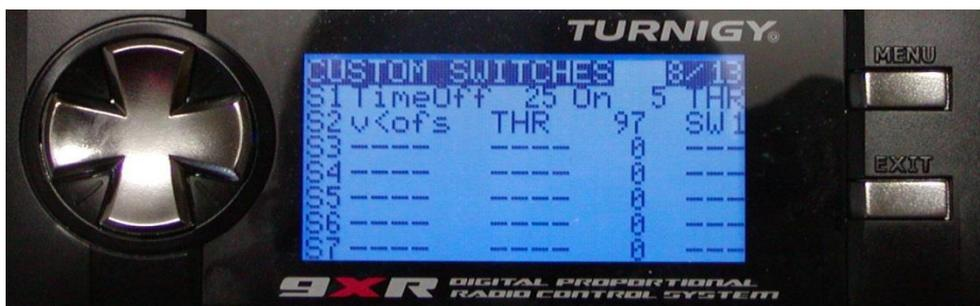
The first "operation" column lists several arithmetic, logical and differential operations. In arithmetical operations, a and b represent variables and x represents a constant. Variables can be any source, i.e., all the available in mixers, plus the five global variables and all telemetry values. In logical operations the available sources are all the physical switches and the other custom switches. Differential functions compare the changes in a variable since last match to another value.
