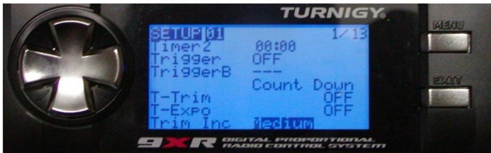
Trigger B options are any physical switch and any virtual switch (more on those later)
