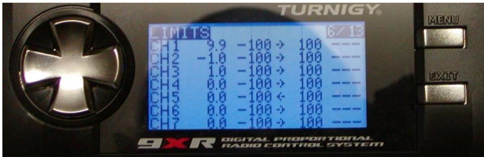
Each channel here corresponds to a channel in the receiver. The limits you set on a line apply to that channel only. Here's what you see in this screen:
