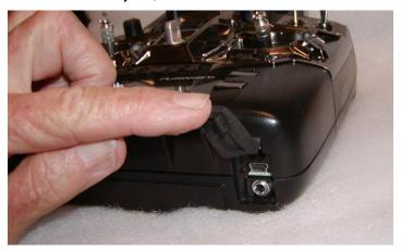
To set up a USB connection between the transmitter and a PC, start with the transmitter turned OFF. Hold both horizontal trim switches (Aileron and Rudder) TOWARDS THE CENTER and turn ON the transmitter. You will see "Boot Loader Ready" on the transmitter screen. From this point on, procedures are different for PCs and Macintosh computers.
