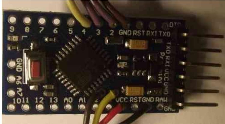
At the top (IO2, IO3 and IO4) are the connections to the encoder. The wire colours are:
